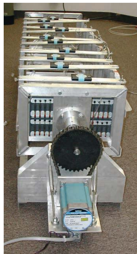
Rough night. This robot periodically jostles vials of fruit flies, keeping the insects awake for sleep-deprivation studies.
